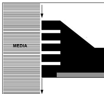
and effective sealing due to the use of four pass labyrinth seal.
