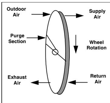
Cross contamination generally refers to a mixing of air between supply and exhaust air streams. In rotary heat exchangers, this occurs through leakage and carryover. Carryover occurs each time a portion of the matrix passes the seals
