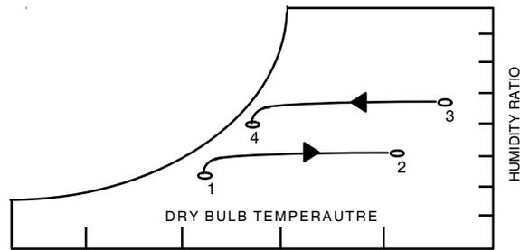
Figure B : Sensible Heat Exchanger Recovering Latent Heat
