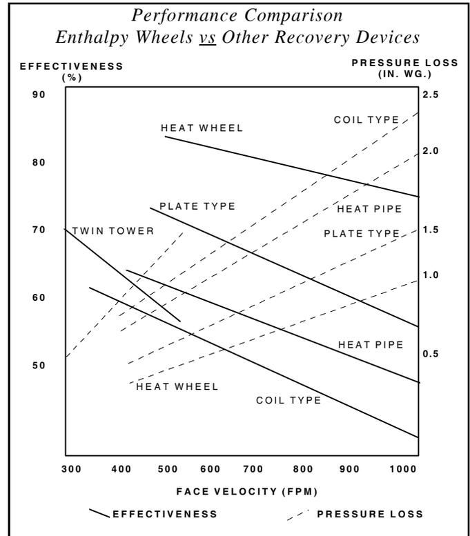
It is seen that the enthalpy wheel has the highest effectiveness and least pressure drop at any face velocity, making it the most appropriate choice for energy recovery in comfort ventilation.
