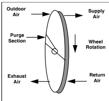
Cross contamination generally refers to a mixing of air between supply and exhaust air streams. In rotary heat exchangers, this occurs through leakage and carryover. Carryover occurs each time a portion of the matrix passes the seals
