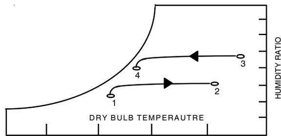
Figure B : Sensible Heat Exchanger Recovering Latent Heat
